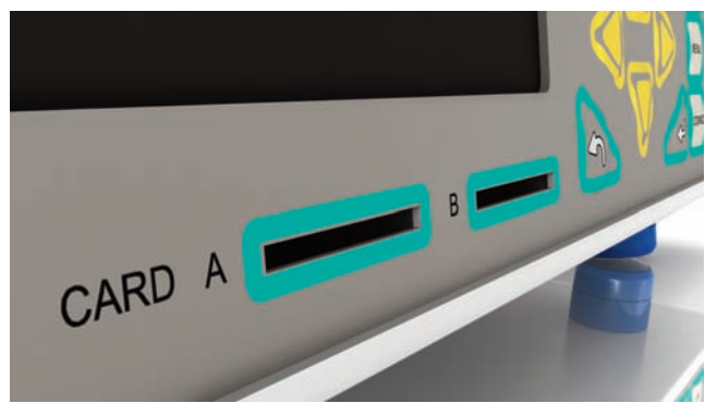
Memory card slots for separate data collection and sequence scripting
